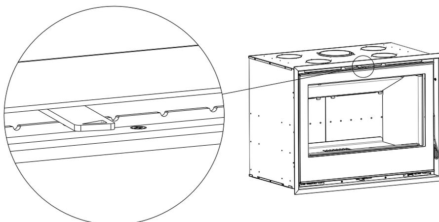
**SECONDARY AIR REGULATION LEVER POSITION FOR NOMINAL POWER, OPEN 25% OF ITS RANGE.**
