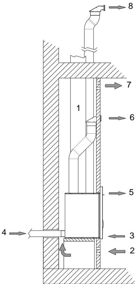
1. Fumes exhaust pipe  $\varnothing$  200 or 150, according to model.
