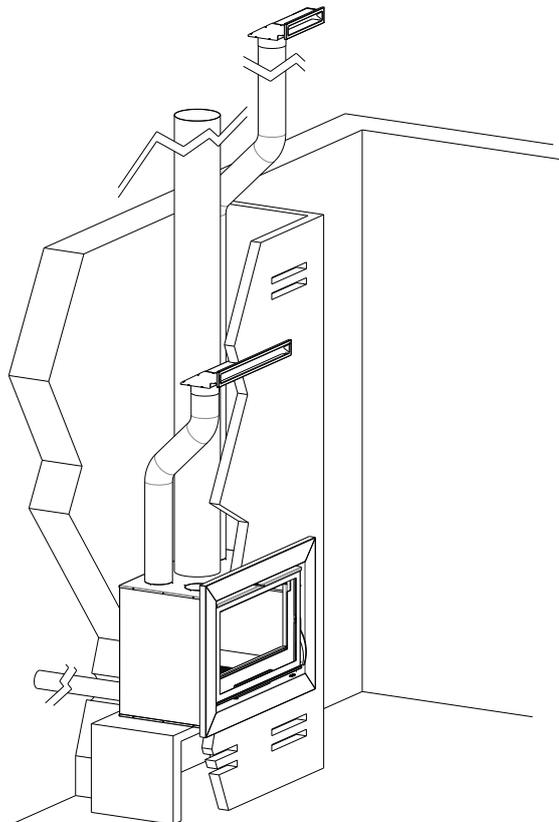
The building work must be finished in such a way that the wood burner can expand during operation: the brickwork must never be supported on or against the sides of the appliance. Leave a minimum expansion joint of 0.5 cm on each side and at least 1 cm the top of the front.
